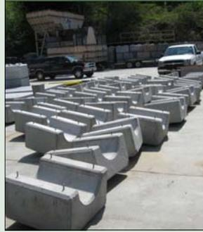
*Precast concrete anchors*
