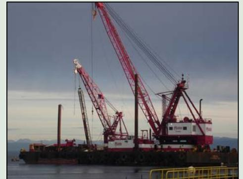
*The derrick barge Viking, which will be used for lake line construction, is 260 feet long and 66 feet wide*
